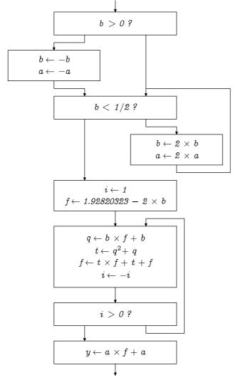
The flowchart is executed in such a way that there are always two iterations. The error is then smaller than  $0.5 \times 10^{-10}$ , which is enough for the precision of the ARMAC.<sup>1</sup>
